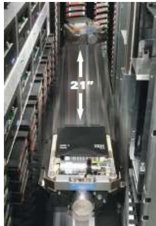
In just 21" of horizontal travel the XLS robot can access over 3,200 tapes.
