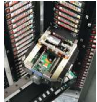
Robotics never leave the LRM to access cartridges in the MEM, insuring fast access times and high reliability.
