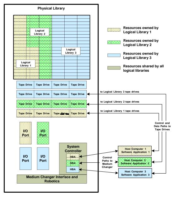
**Figure 5-1** Example configuration showing the relationship between the physical library, logical libraries, and software applications
