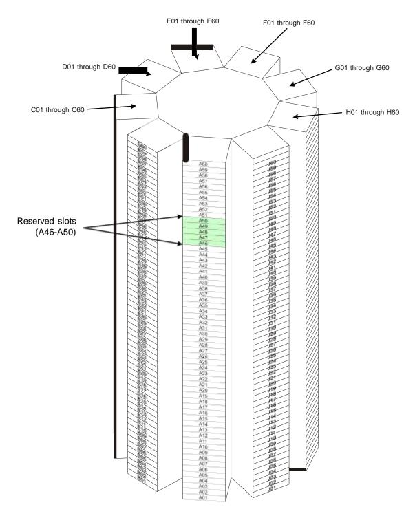
Figure A-18 Physical addresses for the slots in an XLS-85000 Media Expansion Module
