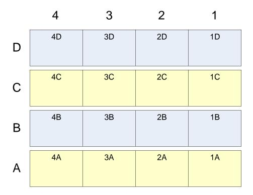
Figure A-3 Physical addresses for the tape drives in the XLS-8161100, as viewed from the back
