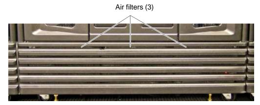
Figure 16-2 Location of the air filters (XLS-832700 shown)
