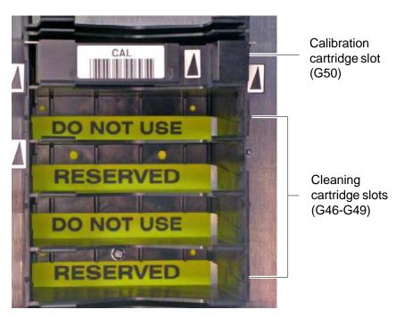
Figure 16-1 Location of the calibration and reserved cleaning cartridges
