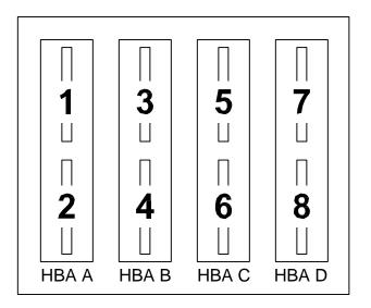
Figure 5-10 HBA port IDs (view from the back of the LRM)
