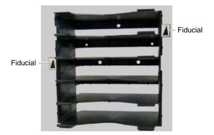
fiducial located on the tape drive calibration cartridge, which is stored in one of the five reserved slots.
