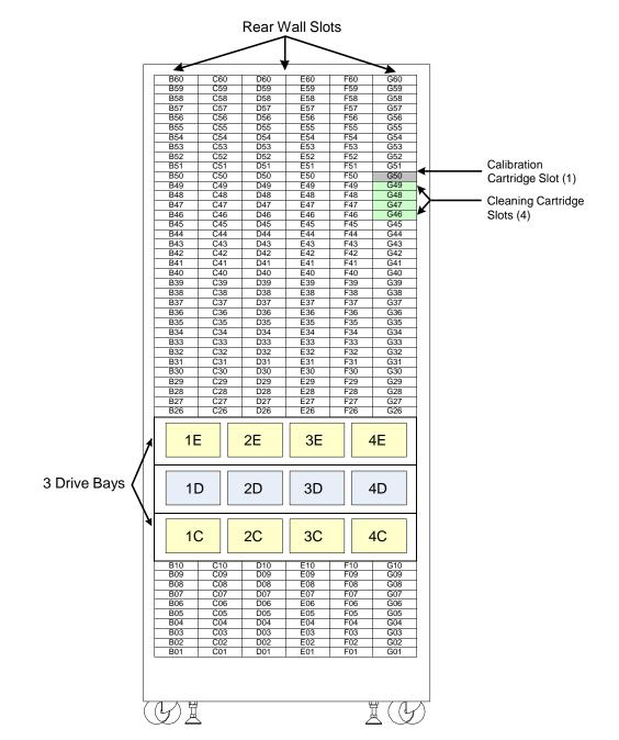
**Figure A-11** Physical addresses for the rear wall of the XLS-812300, with 3 drive bays installed in positions 1C–4E (view from the front with the door open)
