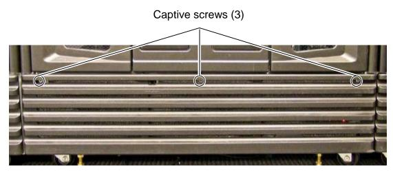
Figure 16-4 Location of the captive screws on the grille (XLS-832700 shown)
