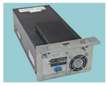
Figure 2-14 Fibre Channel tape drive assembly (rear view)
