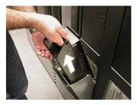
Figure 6-4 Removing the I/O port magazine
