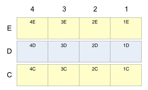
Figure A-12 Physical addresses for the tape drives in the XLS-812300, as viewed from the back
