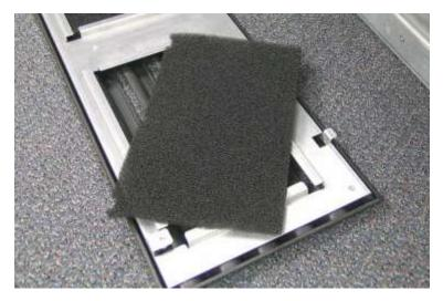
Figure 16-6 Removing the air filter
