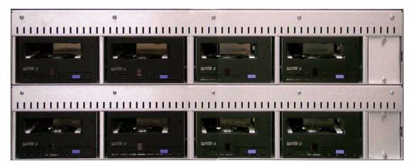
Figure 2-15 Two drive bays (front panel removed)
