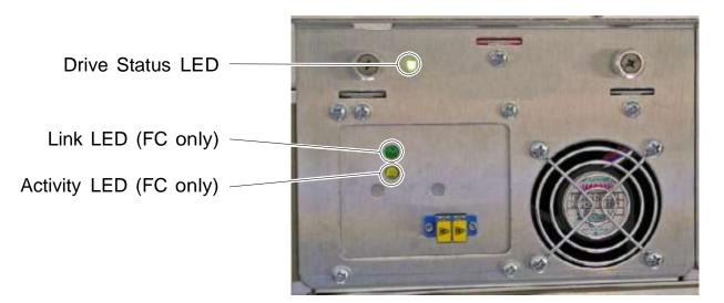
Figure B-3 Status LEDs on Fibre Channel drive carrier
