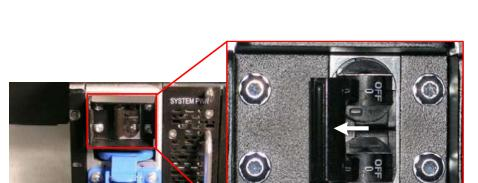
standard power connections or move both switches to the off position for the redundent power input module, as shown in <u>Figure 8-6</u>.
