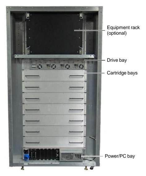
Figure 2-7 Rear view of the LRM (XLS-832700 shown)
