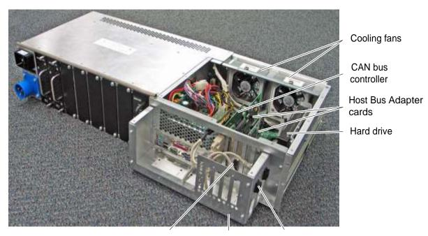
HBA connectors EMI shield Ethernet connectors
