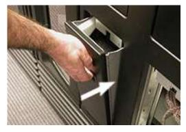
Figure 6-7 Closing the I/O port
