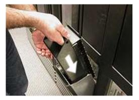
Figure 6-6 Inserting the magazine into an I/O port
