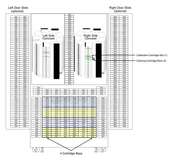
**Figure A-1** Physical addresses for the rear wall and carousels of the XLS-8161100, with 4 cartridge bays installed in positions B01–G20 (view from the front with the doors open)
