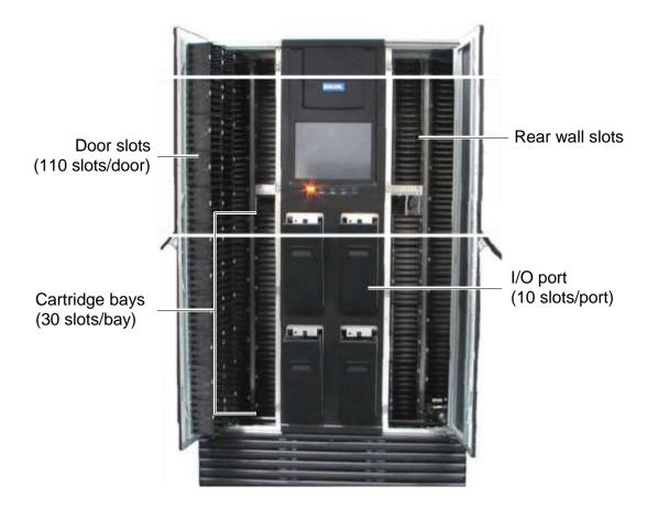
Figure 2-19 Cartridge slots in the XLS-832700 (fixed port slots not shown)
