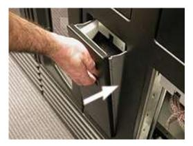
Figure 6-12 Closing the I/O port
