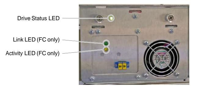
Figure 15-2 Status LEDs on a Fibre Channel tape drive assembly
