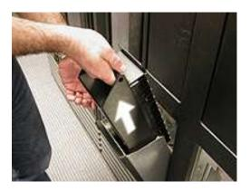
Figure 6-9 Removing the I/O port magazine
