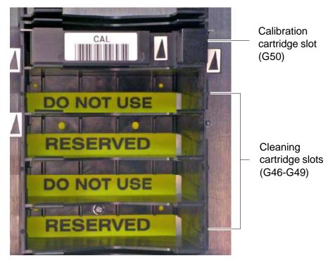
Figure B-10 Location of the reserved slot for the calibration cartridge
