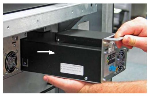
Figure B-5 Removing a drive carrier from a drive bay
