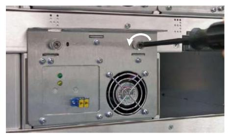
Figure B-4 Loosening the tape drive assembly screws
