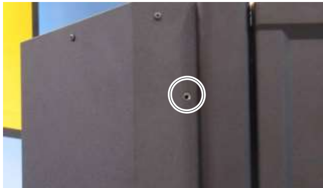
Figure 6-15 Location of top-most hole for securing an expansion pod to the XLS-812300
