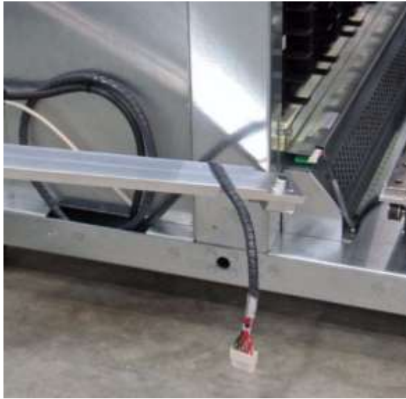
Figure 6-7 Routing the expansion-pod controller cable through the bottom hinge mount
