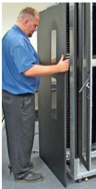
Figure 5-2 Removing a side panel (XLS-832700 shown)
