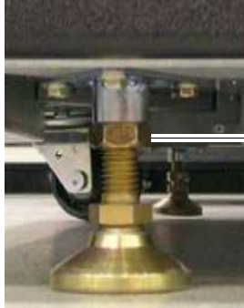
Figure 5-17 Tightening a leveling foot
