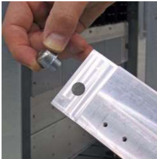
Figure 6-5 Inserting an alignment pin into a hinge mount
