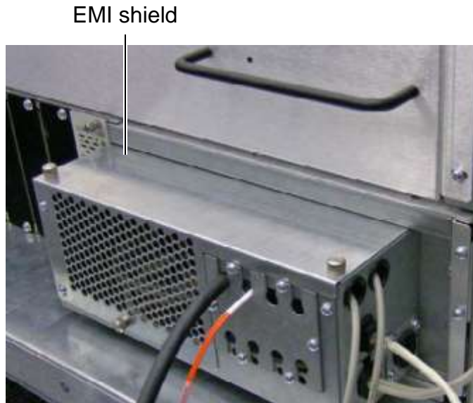
Figure 9-1 Location of the EMI shield (cables shown attached)
