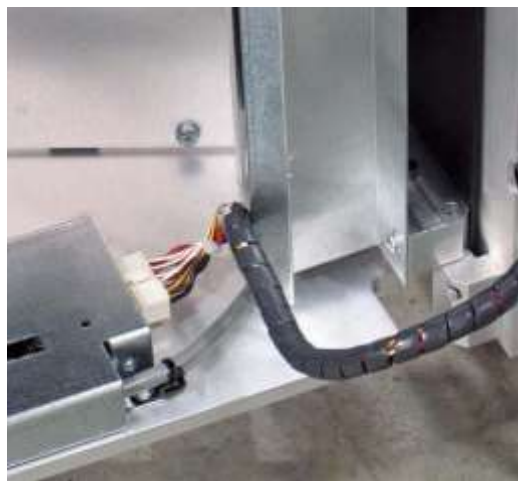
Figure 6-13 Connecting the expansion-pod controller cable to the pod controller
