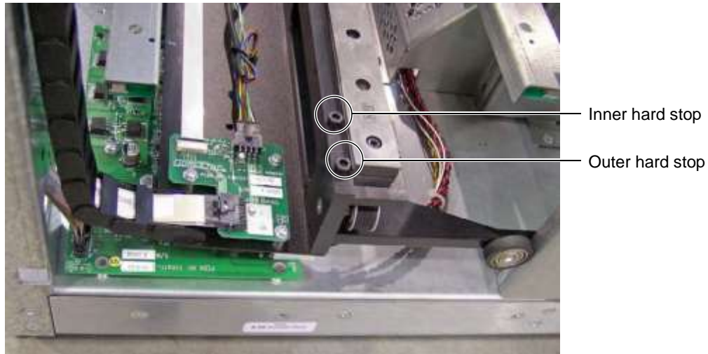
Figure 11-12 Outer and inner hard stops on the handler's X-axis (right side shown)
