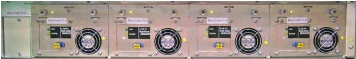
Figure 8-1 Drive bay with four Fibre Channel tape drive assemblies (view from the back)
