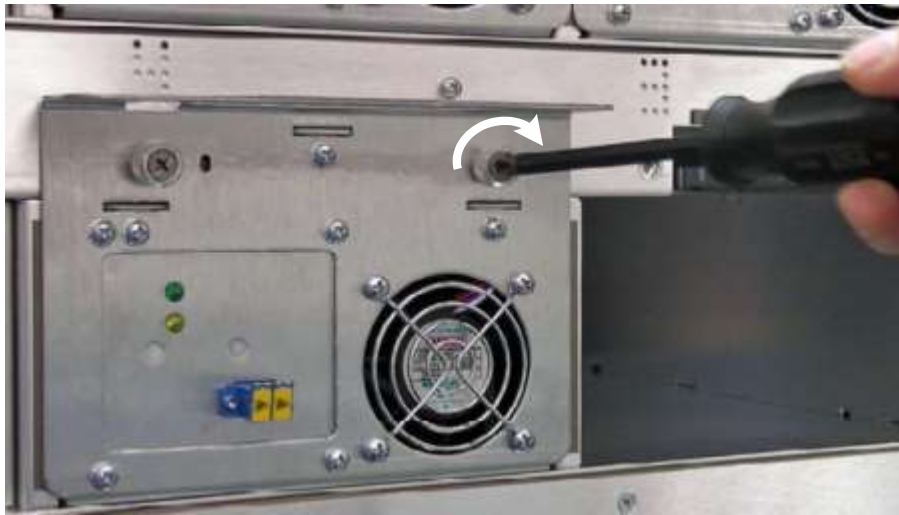
Figure 8-12 Tightening the tape drive assembly screws
