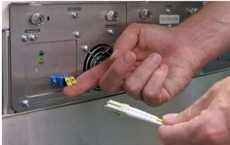
Figure 9-4 Attaching the cable to a Fibre Channel tape drive
