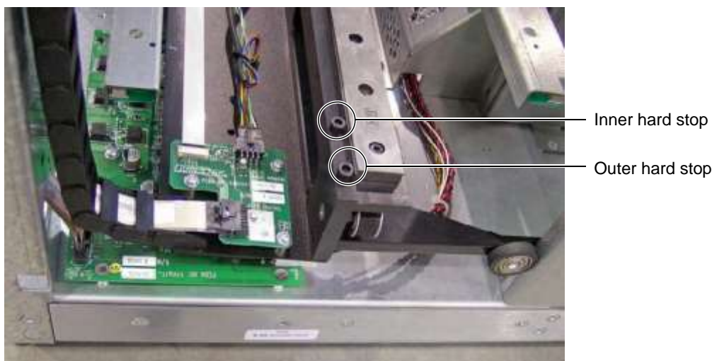
Figure 5-4 Outer and inner hard stops on the handler's X-axis (right side shown)
