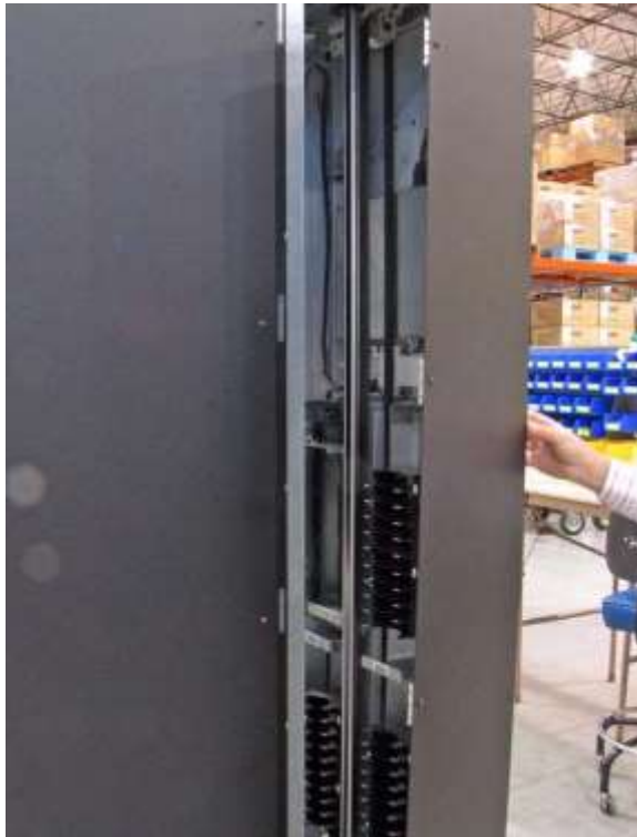
Figure 6-2 Removing the front side panel
