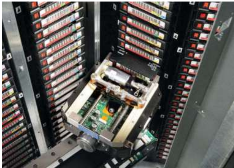
Figure 1-12 Robotic handler (shown reaching into an attached MEM)
