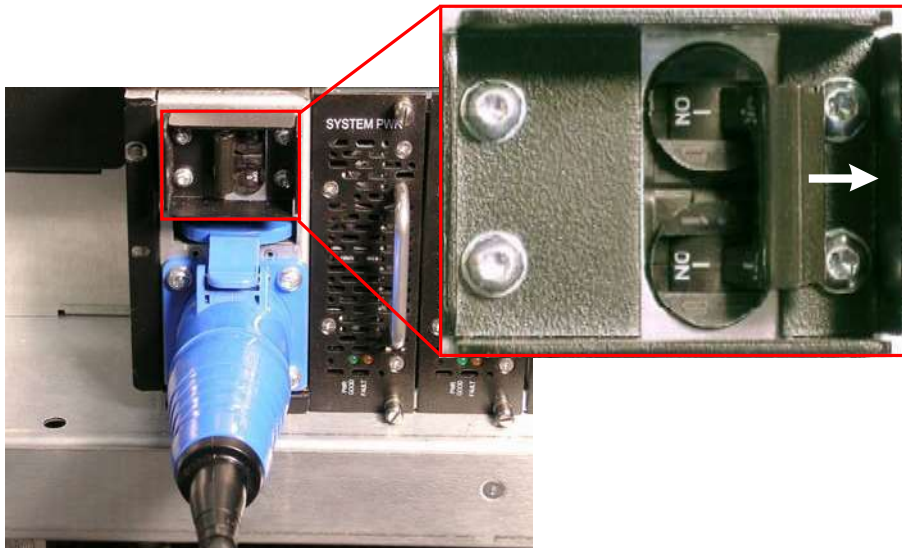
Figure 10-3 Power switch in on position
