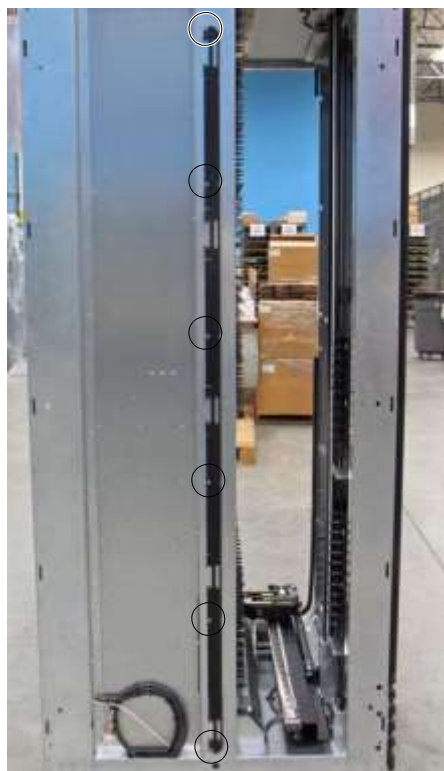
Figure 6-3 Removing the center mounting rail from the side of the XLS-812300
