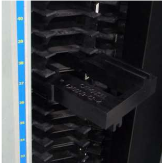
Figure 11-8 Inserting the gripper alignment cartridge into the carousel
