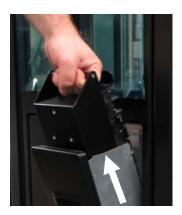
**Figure 6-13** Removing the I/O port magazine
