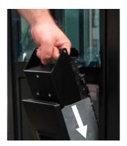
**Figure 6-6** Inserting the magazine into an I/O port
