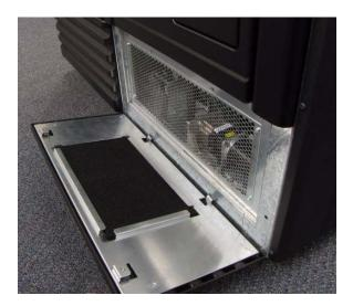
Figure 16-5 Releasing the top edge of the grille
