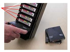
Figure 6-9 Inserting cartridges into the I/O port magazine
