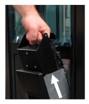
**Figure 6-8** Removing the I/O port magazine
