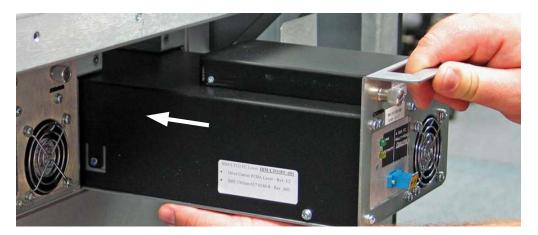
Figure B-6 Inserting a tape drive assembly into a drive bay
