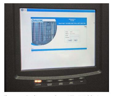
Figure 2-7 Touch screen and status LEDs (X-Link log-in screen displayed)
