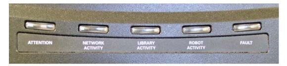
Figure 15-1 Status LEDs on the LRM front panel
