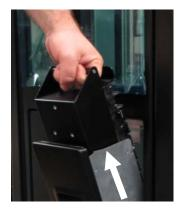
**Figure 6-4** Removing the I/O port magazine
