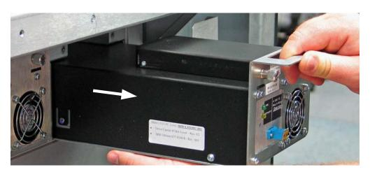
**Figure B-5** Removing a drive carrier from a drive bay
