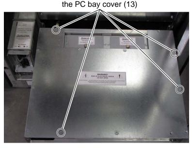
Figure 16-8 The screws that attach the PC bay cover
