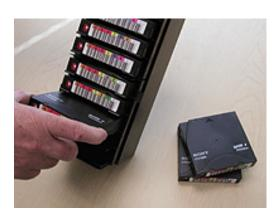
Figure 6-14 Removing cartridges from the I/O port magazine
