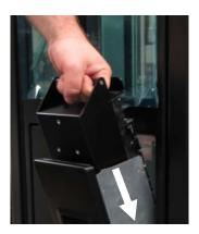
Figure 6-10 Inserting the magazine into an I/O port
