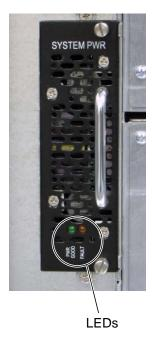
**Figure 15-3** Power supply LEDs
