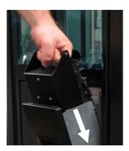
Figure 6-15 Inserting the magazine into an I/O port
