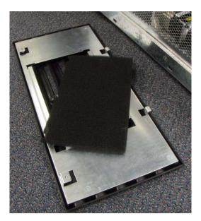
**Figure 16-6** Removing the air filter
