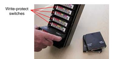
**Figure 6-5** Inserting cartridges into the I/O port magazine
