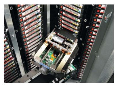
Figure 2-9 Robotic handler (shown reaching into an attached MEM)
