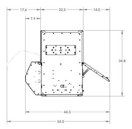
Figure 3-2 Service access requirements for the XLS-810160/810240, including expansion pod
