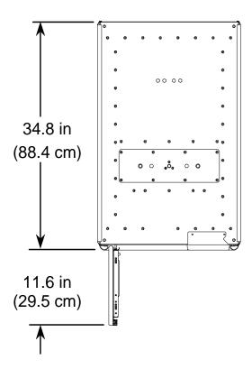
Figure 3-4 Service access requirements for a XLS-85000 MEM2
