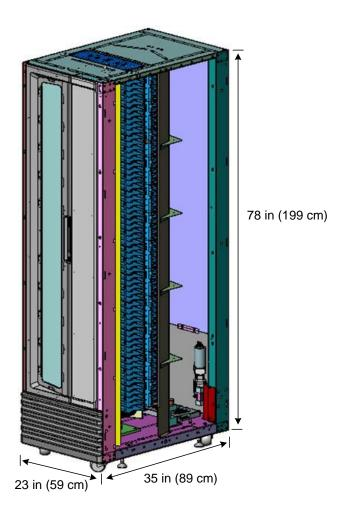
Figure 3-3 External dimensions of the XLS-85000 MEM2
