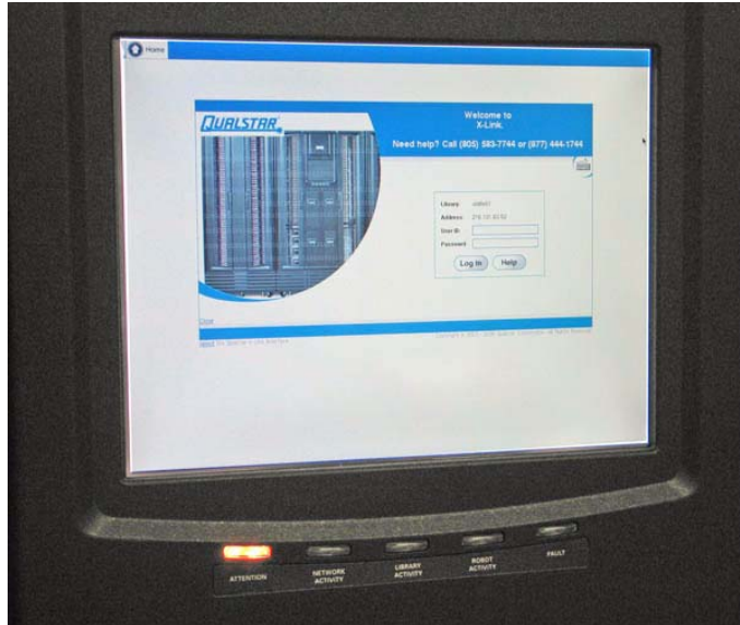
Figure 1-7 Touch screen and status LEDs (X-Link log-in screen displayed)
