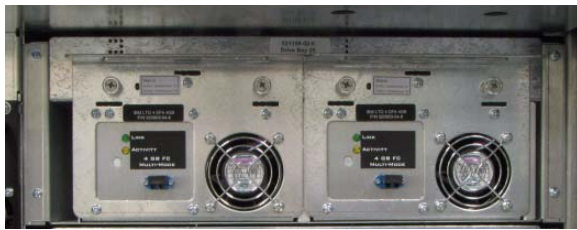
Figure 7-1 Drive bay with two Fibre Channel tape drive assemblies (view from the back)
