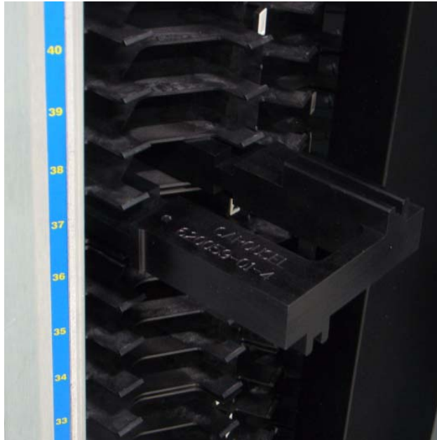
Figure 10-8 Inserting the gripper alignment cartridge into the carousel
