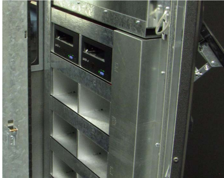
Figure 1-12 View of drive bays through the open door
