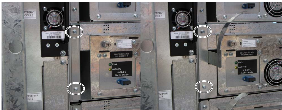
Figure 8-5 Attaching the cable routing brackets
