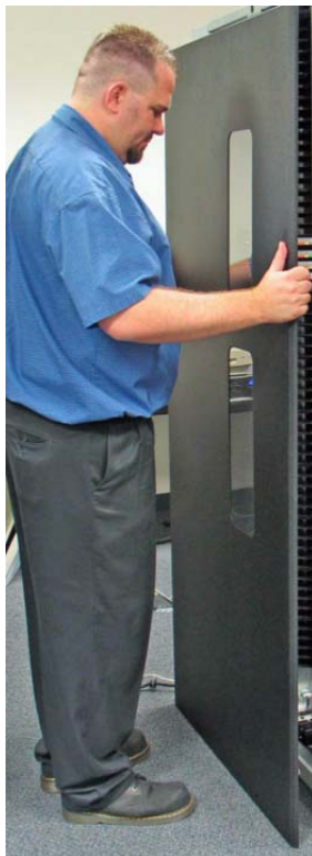
Figure 5-2 Removing a side panel
