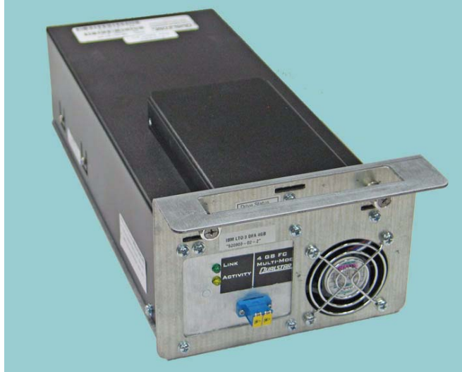
Figure 1-11 Fibre Channel tape drive assembly (rear view)
