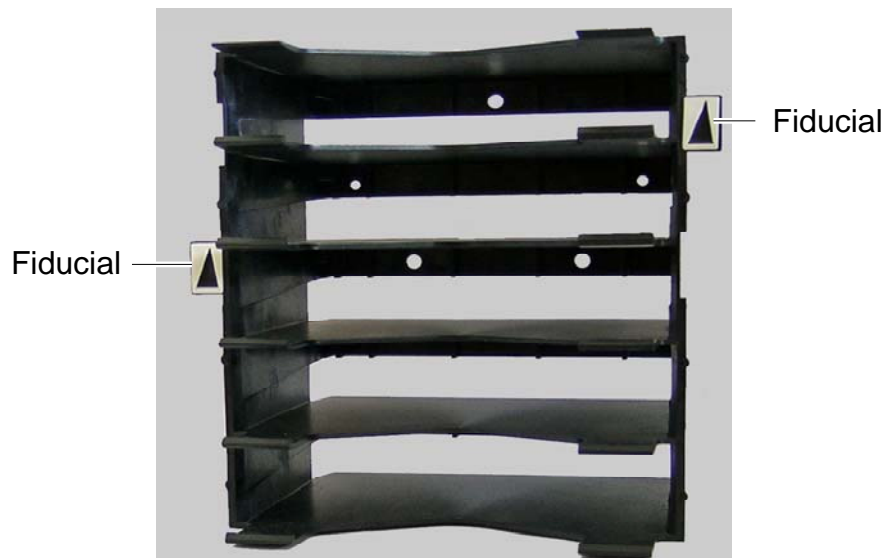
Figure 13-1 Cartridge magazine with two fiducials
