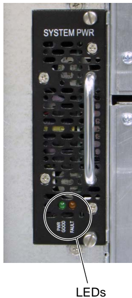
Figure 9-8 Power supply status LEDs
