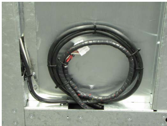
Figure 5-3 Carousel controller cable on the side of the LRM
