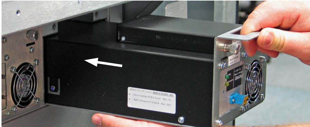
Figure 7-11 Inserting a tape drive assembly into a drive bay
