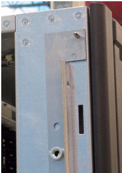
Figure 6-8 Front L brace on the left side of the LRM
