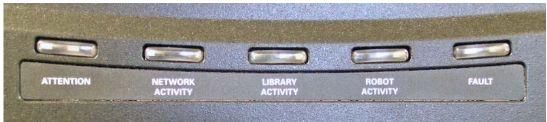
Figure 9-6 Status LEDs on the LRM front panel
