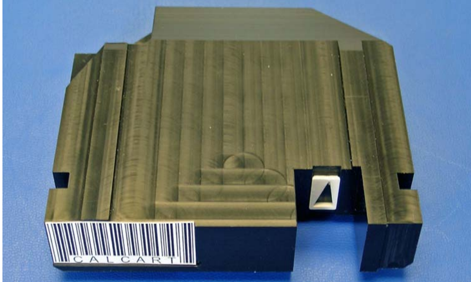
Figure 12-1 XLS calibration cartridge
