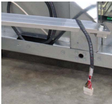
Figure 6-6 Routing the expansion-pod controller cable through the bottom hinge mount
