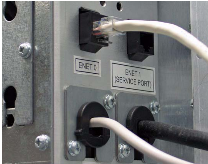
Figure 10-1 Location of the primary Ethernet connector
