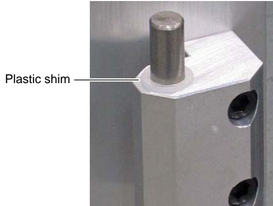
Figure 6-7 Installing a plastic shim on a hinge pin
