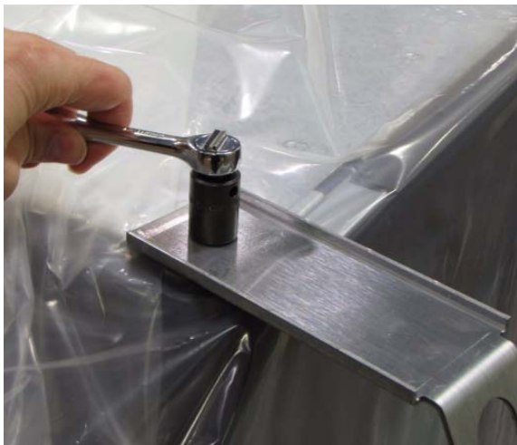
Figure 3-5 Removing a shipping bracket
