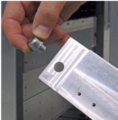
Figure 6-4 Inserting an alignment pin into a hinge mount
