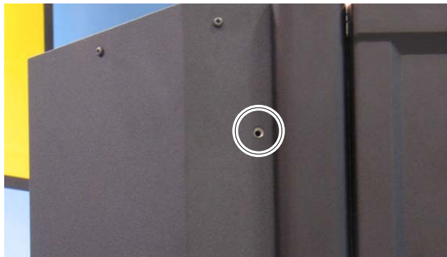
Figure 6-14 Location of top-most hole for securing an expansion pod to the XLS-810160/810240
