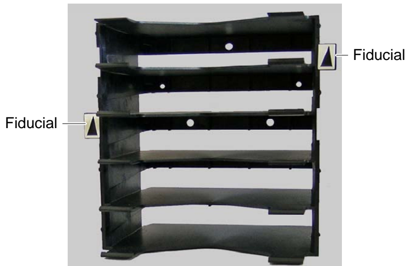
Figure 1-10 Cartridge magazine with two fiducials
