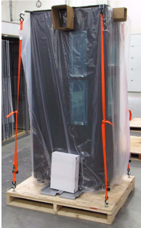
Figure 3-3 LRM with crating material removed
