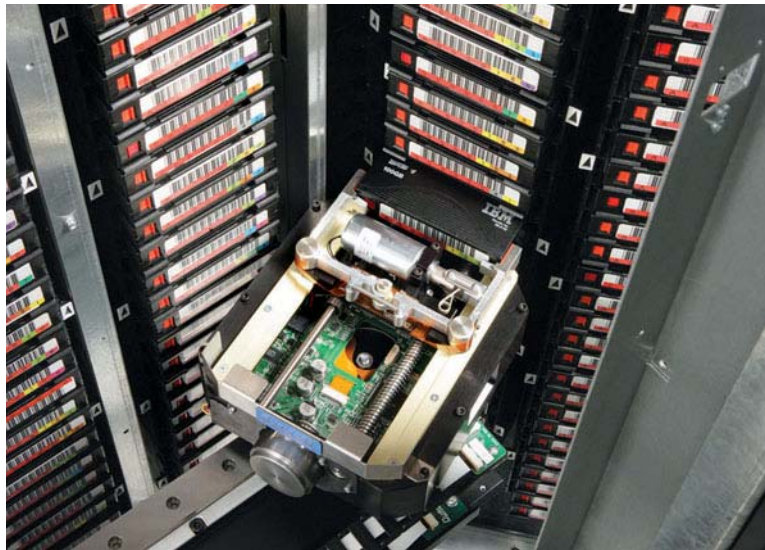
Figure 1-9 Robotic handler (shown reaching into an attached MEM)
