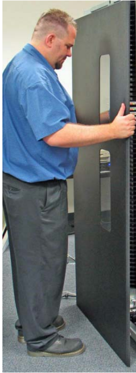
Figure 6-2 Removing a side panel
