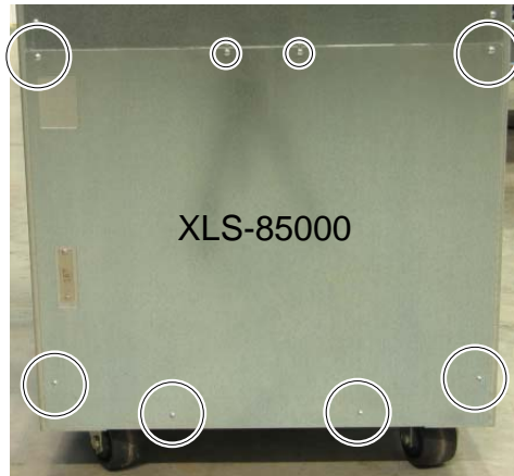
Figure 5-8 Removing the MEM's lower back panel
