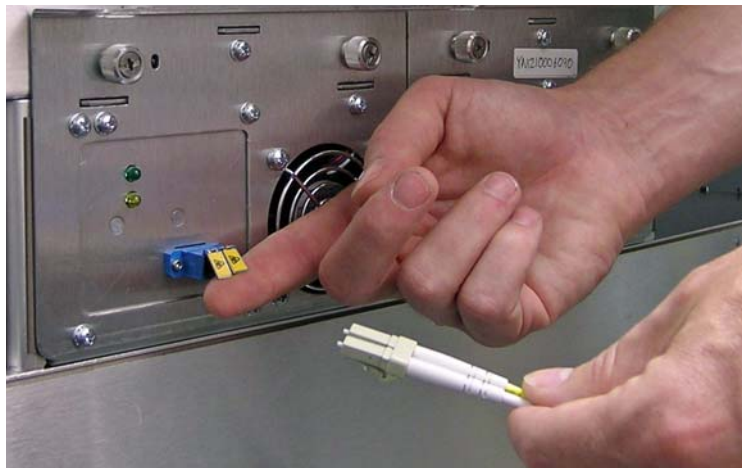
Figure 8-4 Attaching the cable to a Fibre Channel tape drive
