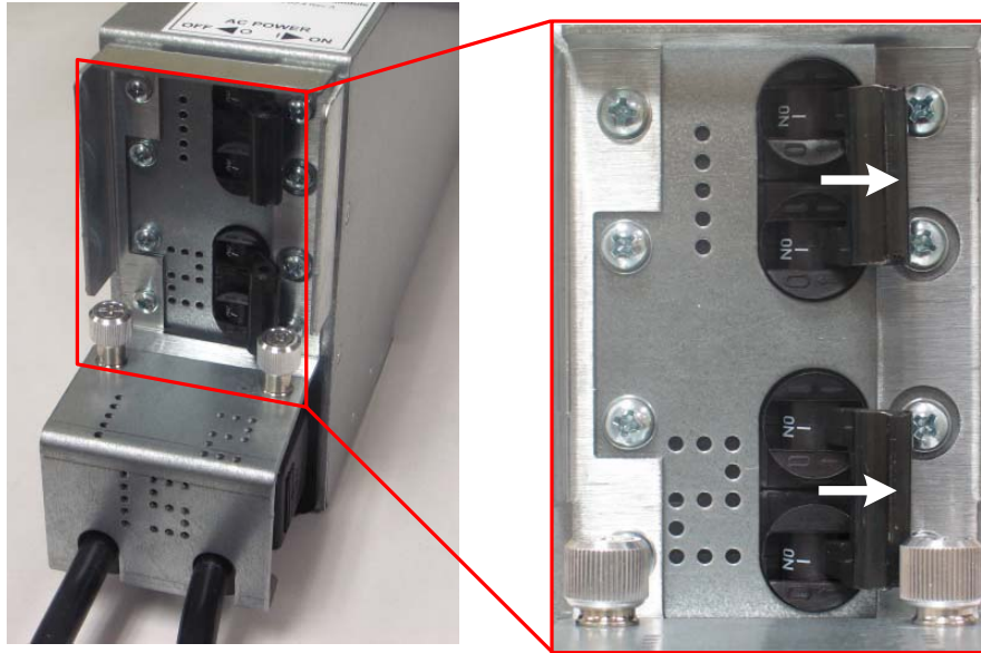
Figure 9-5 Power switches in the on position
