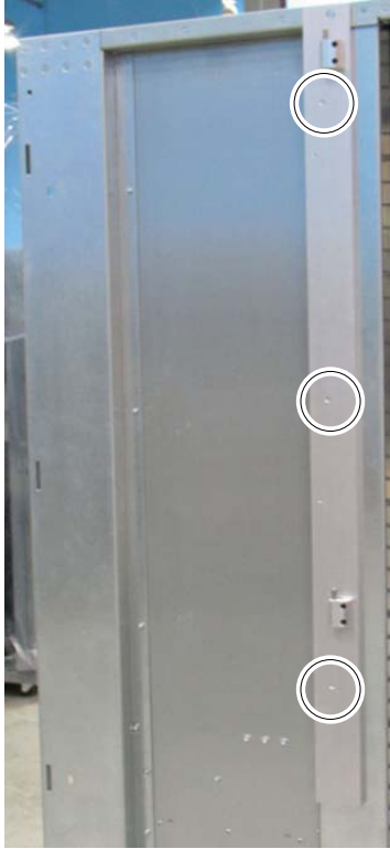
Figure 6-5 Attaching the top hinge mount
