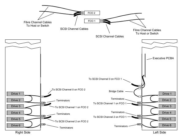
Figure 5-7 TLS-412xxx Cabling Diagram for up to 12 AIT-5 Tape Drives
