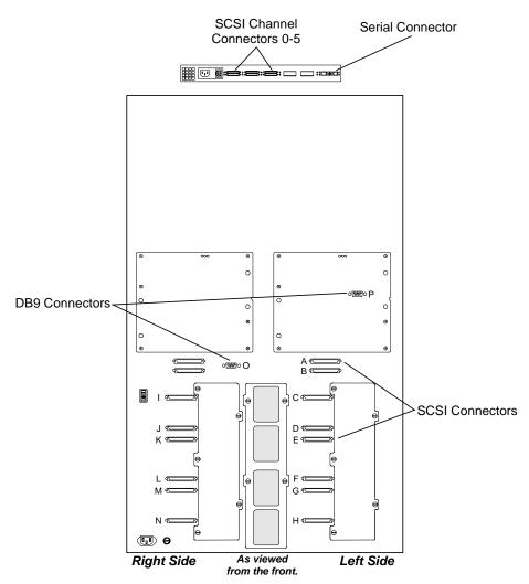
Figure 5-4 Connector Locations on the Rear of the TLS-412xxx
