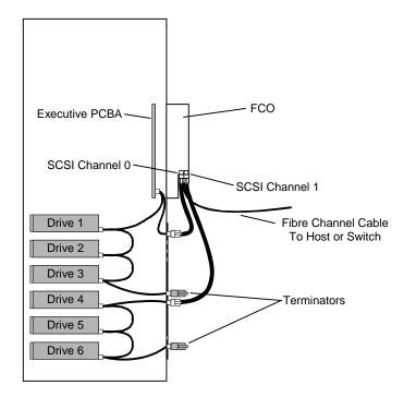
Figure 4-4 TLS-46xxx Cabling Diagram using AIT-3 Tape Drives
