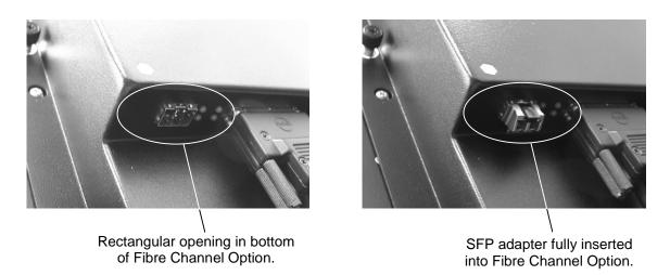
Figure 4-16 Inserting SFP Adapter into Fibre Channel Option
