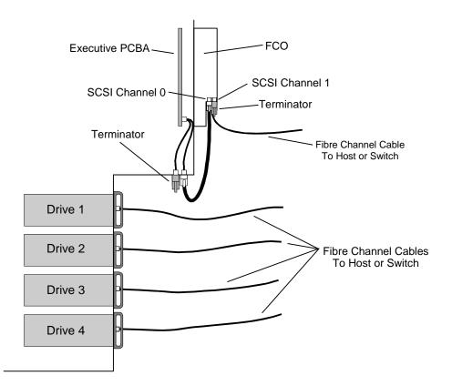
Figure 4-6 TLS-84xx Cabling Diagram
