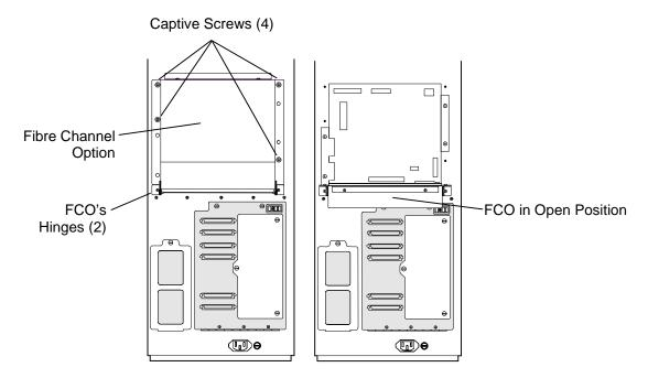
Figure 9-2 Fibre Channel Option in Closed and Open Positions
