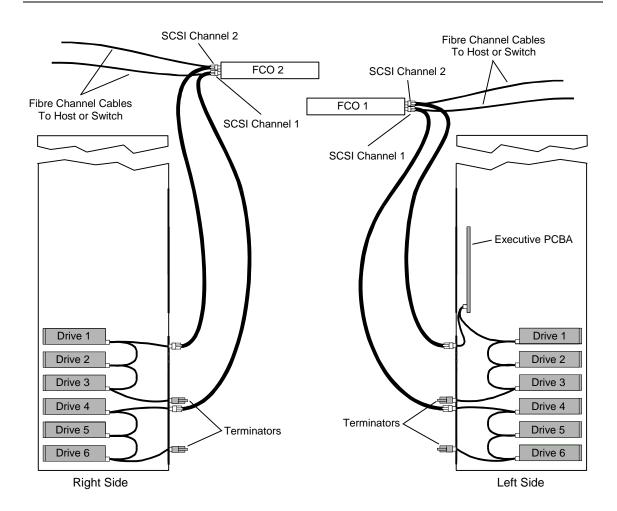
Figure 6-5 TLS-412xxx Cabling Diagram for up to 12 AIT Tape Drives
