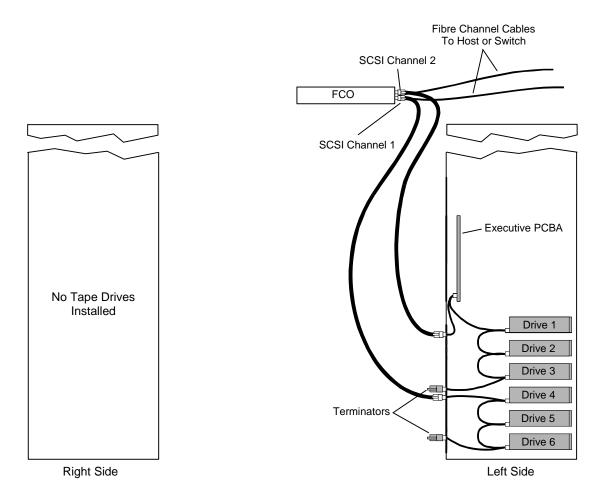
Figure 6-4 TLS-412xxx Cabling Diagram for up to 6 AIT Tape Drives
