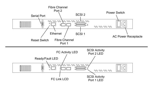
Figure 9-6 Rear View of the ATTO Fibre Channel Bridge/Router (FCO)
