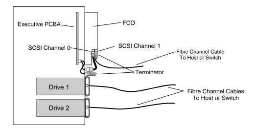
Figure 4-5 TLS-82xx Cabling Diagram
