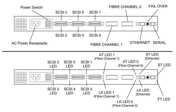
Figure 5-1 Rear View of the Type B Fibre Channel Bridge/Router (FCO)
