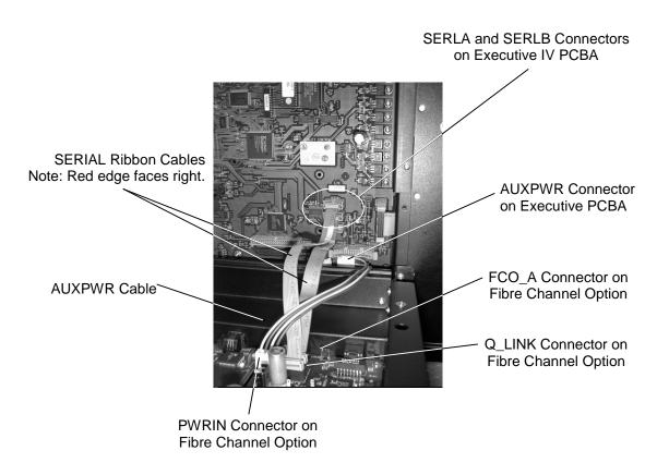
Figure 4-13 Detail of Connections (Executive IV PCBA Shown)
