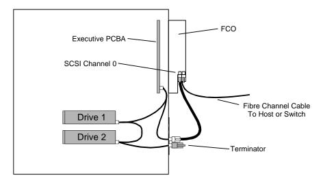
Figure 4-2 TLS-42xx Cabling Diagram
