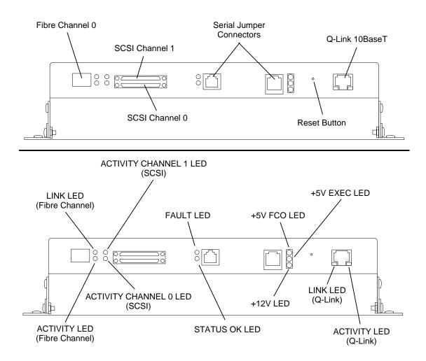
Figure 4-1 Bottom View of the Type C Fibre Channel Bridge/Router (FCO)
