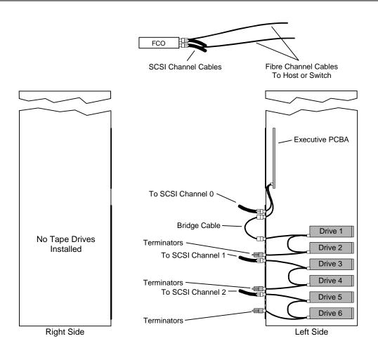
Figure 5-6 TLS-412xxx Cabling Diagram for up to 6 AIT-5 Tape Drives
