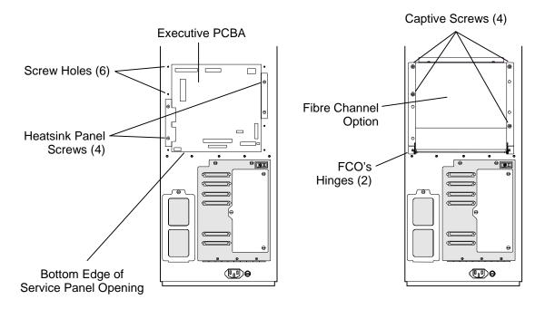
Figure 4-9 Rear View of TLS
