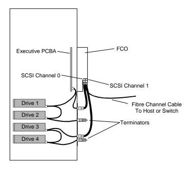
Figure 4-3 TLS-44xx Cabling Diagram using AIT-3 Tape Drives
