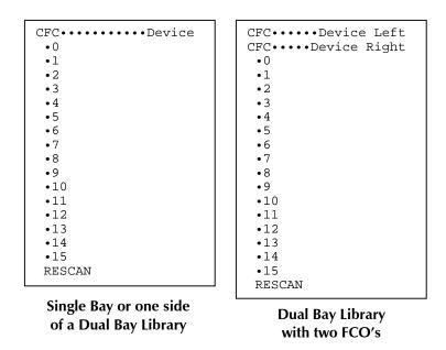
The Fibre Channel Option assembles a list of SCSI devices it detects on its three SCSI channels. This menu displays the SCSI devices that a Fibre Channel Option has detected. To initiate the scan operation, press the (DOWN) key to move the pointer to RESCAN and press the ENTER key. The RESCAN item will disappear and return when the operation completes.
