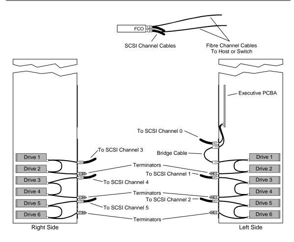
Figure 5-5 TLS-412xxx Cabling Diagram for 12 AIT-3 Tape Drives
