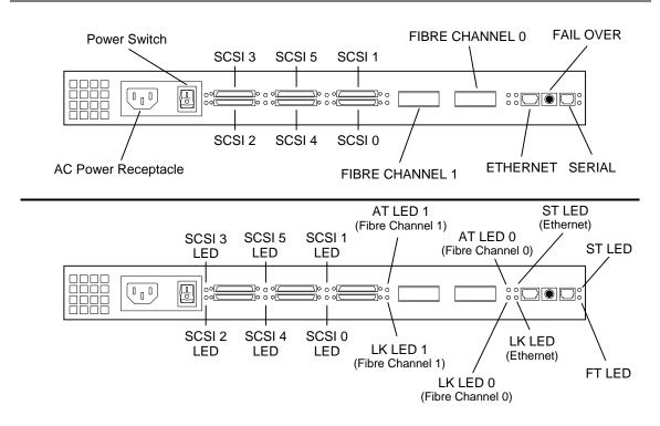
Figure 9-5 Rear View of the Type B Fibre Channel Bridge/Router (FCO)
