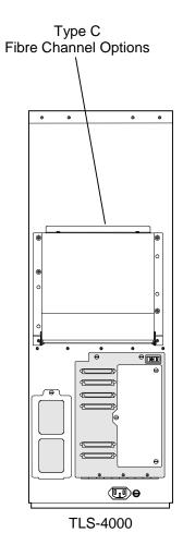
Figure 3-1 Type C Fibre Channel Option Installed on a TLS-4000 Library
