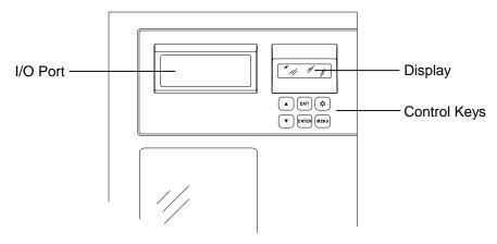
Figure 6-1 TLS Control Panel
