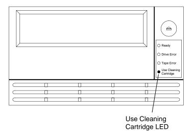
Figure 12-8 HP LTO Tape Drive – Front View
