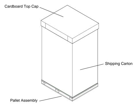
Figure 2-5 Pallet Assembly and Shipping Carton
