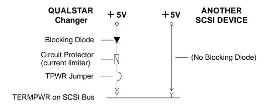
Figure 5-20 SCSI Termination Power Diagram
