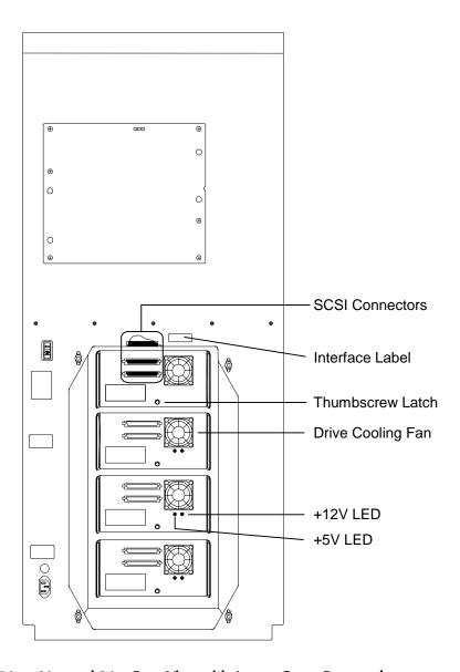
Figure 3-6 54xx, 64xx and 84xx Rear View with Access Cover Removed
