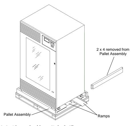
Figure 2-8 2 x 4 Removed and Ramps Under the Library
