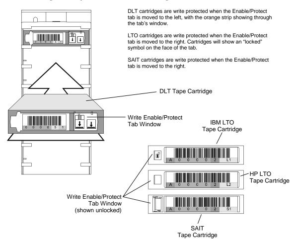
Figure 5-16 Loading a Cartridge Magazine (DLT magazine shown)
