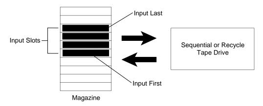
Figure 10-1 Sequential or Recycle Configuration Example
