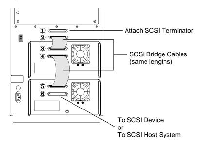
Figure 5-18 SCSI Basic Connection - Model 6220 Shown
