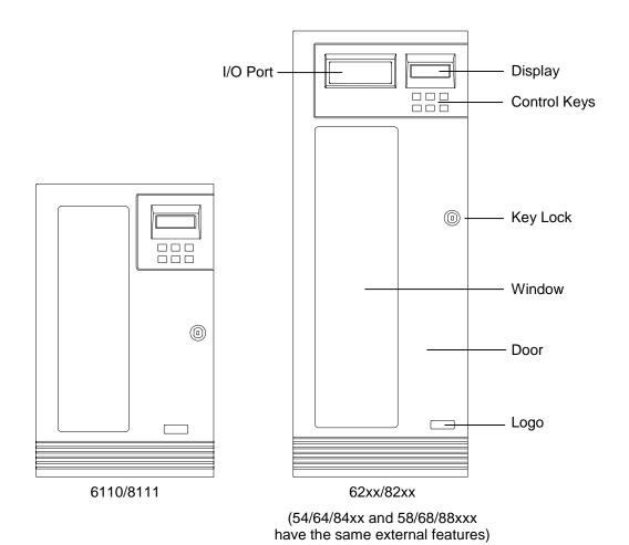
Figure 3-3 TLS Front View
