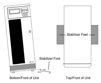
Figure 5-4 Stabilizer Foot Installation
