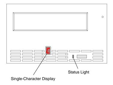
Figure 12-9 IBM LTO Tape Drive – Front View
