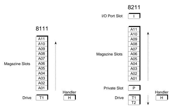
Figure 3-19 8111 and 8211 Cartridge Location Designators
