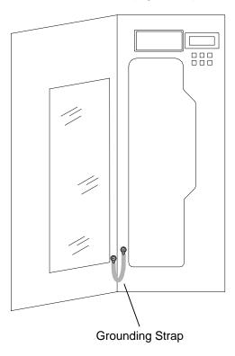
Figure 5-15 TLS Grounding Strap
