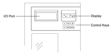
Figure 4-1 TLS Control Panel
