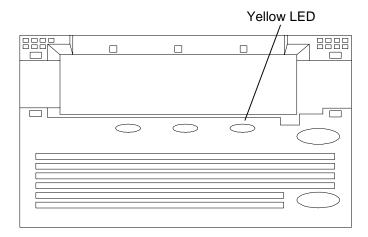
Figure 12-5 Quantum SDLT 320 Tape Drive - Front View
