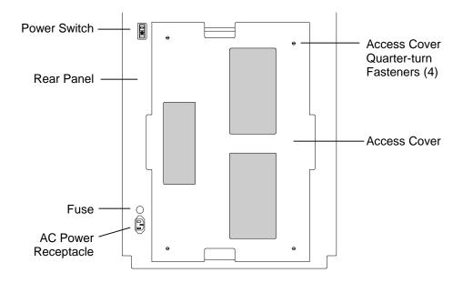
Figure 5-10 TLS Rear View – Model 6430 Shown
