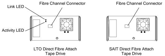
The Direct Fibre Attach Tape Drives require commonly available LC Duplex Multimode fibre channel cables.
