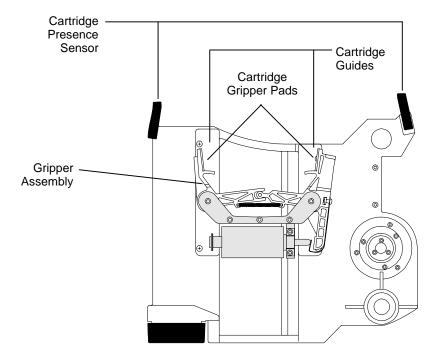
Figure 12-1 The Carriage - Cartridge Presence Sensor and Gripper
