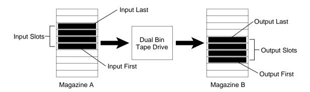
Figure 10-2 Dual-Bin Configuration Example
