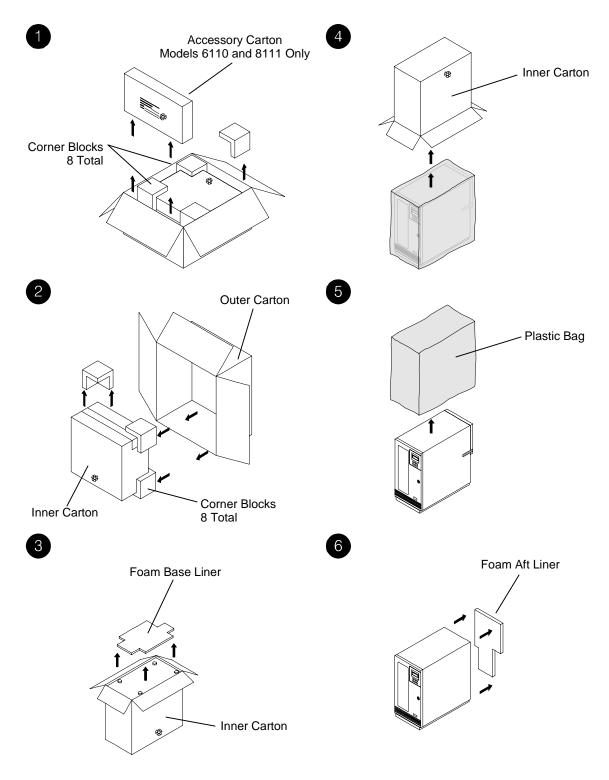
Figure 2-1 Unpacking the TLS - Models 6110, 62xx, 8111 and 82xx
