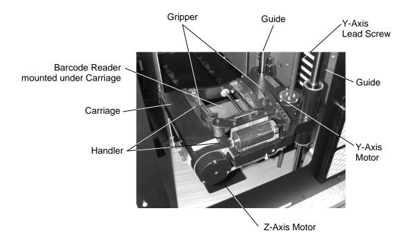
Figure 3-12 The Parts of the Robotics
