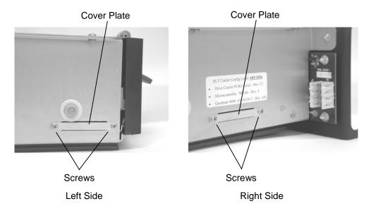
Figure 5-12 Cover Plates in the Closed Position (DLT 4000, 7000 and 8000 Tape Drives Only)
