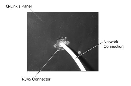
Figure 11-1 Detail of Network Connection Attached to Q-Link
