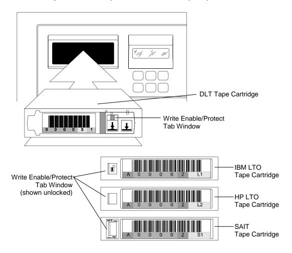
Figure 6-3 Inserting a Tape Cartridge into the I/O Port
