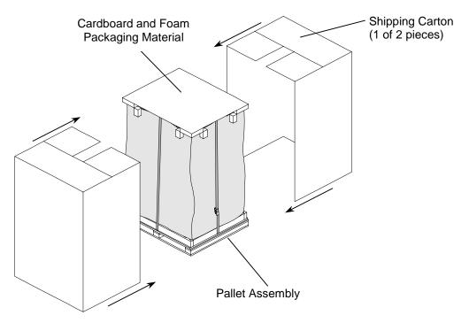
Figure 13-7 Attaching the Shipping Carton to the Pallet Assembly
