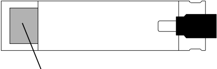
Small circuit board is facing up when oriented correctly for insertion.
