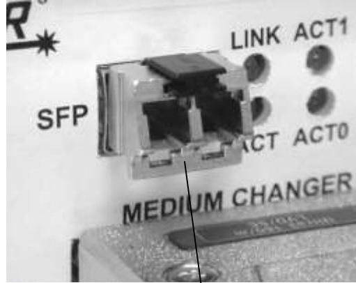
SFP adapter fully inserted into the Fibre Channel Bridge IPM
