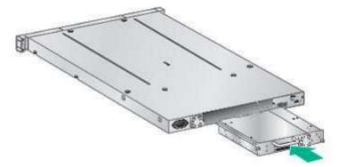
Figure 17 Install a tape drive
