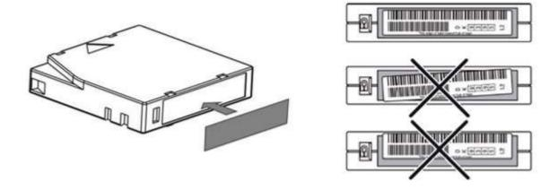
Figure 21 Proper barcode label placement
