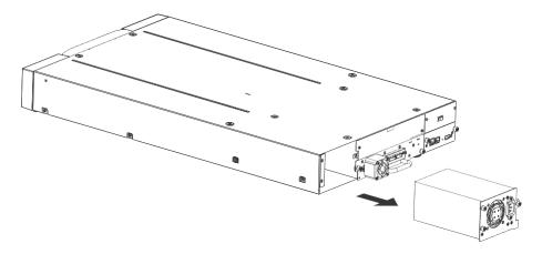
Figure 66 Remove the power supply
