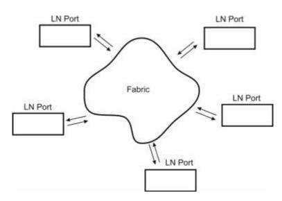
Figure 7 Fibre Channel topology (LN Port)
