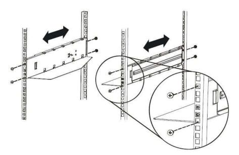
Figure 13 Install the rack rails
