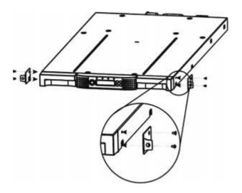
Figure 14 Install the mounting brackets
