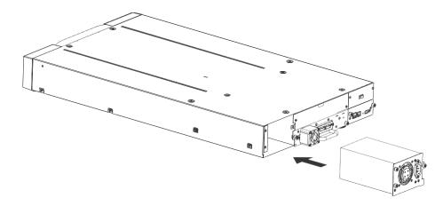
Figure 19 Install a power supply
