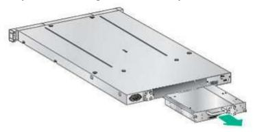
Figure 64 Remove a tape drive
