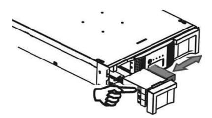
Figure 59 Removing a stuck tape
