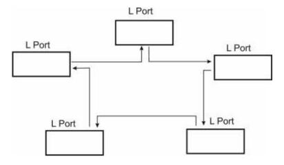
Figure 8 Fibre Channel topology (L Port)
