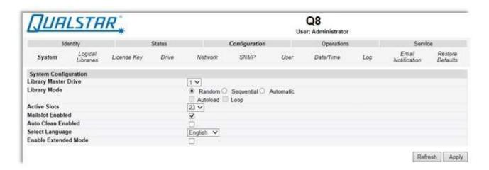
Figure 40 System Configuration
